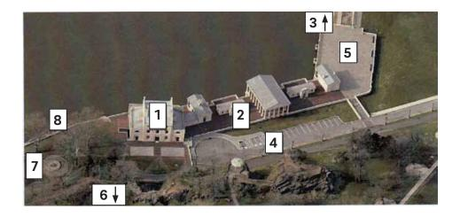
**2.** Old Mill House: Built in 1821-22, in the neoclassical style, it contained eight waterwheels. In 1872, the Old Mill house was altered to provide room for the turbines. When it was remodeled again for the Aquarium in 1911, all pumping machinery was removed to accommodate the fresh water exhibits. The red brick desk is actually the roof of the building upon which rest the five smaller structures described below.
